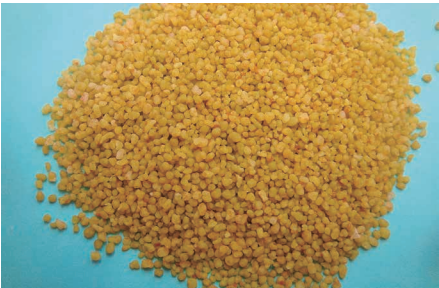
Food Granulation of high-density or porous structure d=200 μm~5 mm e.g. instant beverage, soup powder
