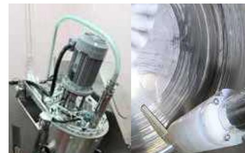
EIRICH Smart Discharger (ESD), suction-type product discharge device
