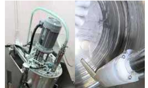
EIRICH Smart Discharger (ESD), suction-type product discharge device
